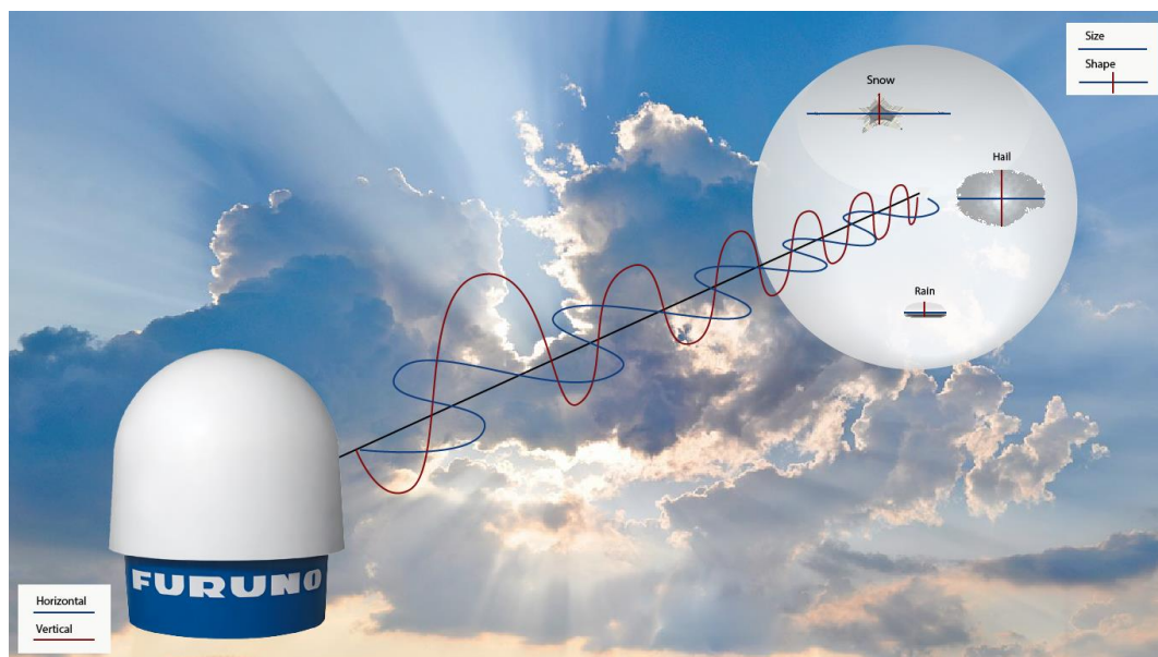
Fig. 3 Dual polarization of electromagnetic waves used in meteorological radars [WR-2120, 2024].
