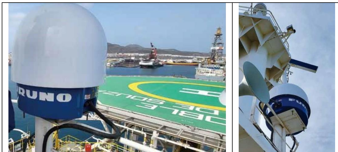
Fig. 9. WR 2120 weather radar used on the oil rig and the drilling ship [Compact X-band Dual Polarimetric Doppler Weather Radar, p. 5].
