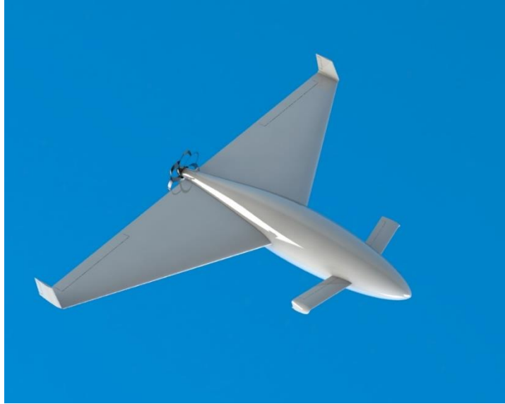
Fig. 4. Main and auxiliary wings of the demonstrator model
