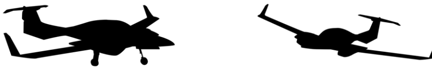
Fig. 8. Comparison of DA42 type in two landing gear configurations. On the left: DA42 with landing gear deployed. On the right: DA42 with landing gear retracted.
