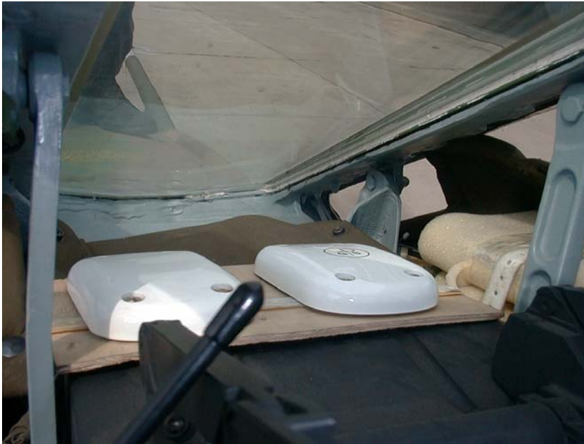
Fig. 1. Mounting the satellite receiver antennas in Su-22M4 aircraft cockpit (25 th April.1999.)
