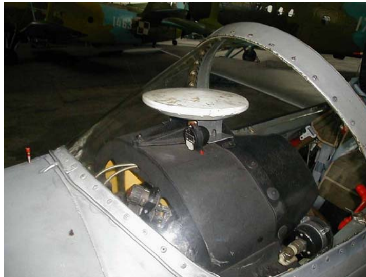
Fig. 25. Assembly of GPS antenna onboard the TS-11 Iskra aircraft
