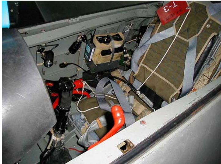
Fig. 26. Assembly of the GPS receiver and the radio modem onboard the TS-11 Iskra aircraft
