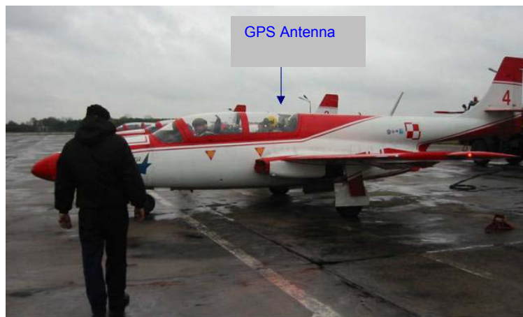
Fig. 39. Location of the GPS antenna during experimental flights.
