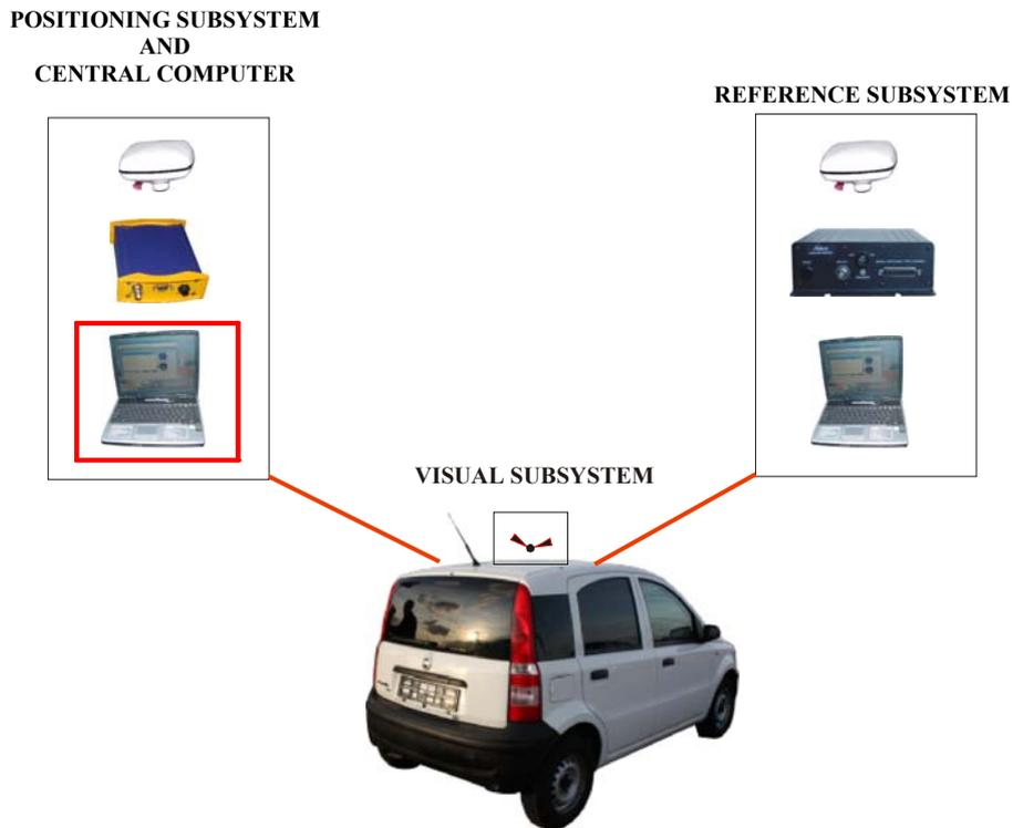
Fig. 2. The architecture of mobile measurement station
