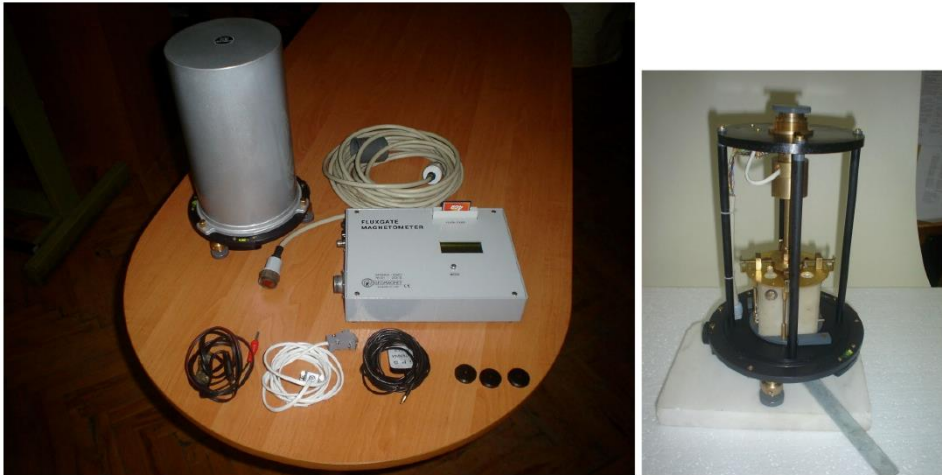
Fig. 4. Flux-gate magnetometer to be used in marine measurements. (Source: Marianiuk J. et al., 2007)
