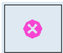
Fig. 3. Isolated danger of depth less than the safety contour: wrecks, obstructions, under water rocks [source: IHO publication S-52 Appendix 2 Addendum to Annex 2, Part I, Users' Manual Edition 3.4 2008]
