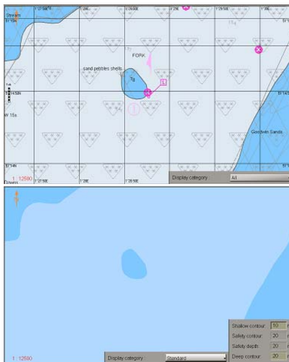
Fig. 4. Extract from ECDIS 3000-i showing alternative display settings for ENC charts for area in question: a) wreck visible, b) wreck not visible (improper setting: shallow and deep contour) [own study]
