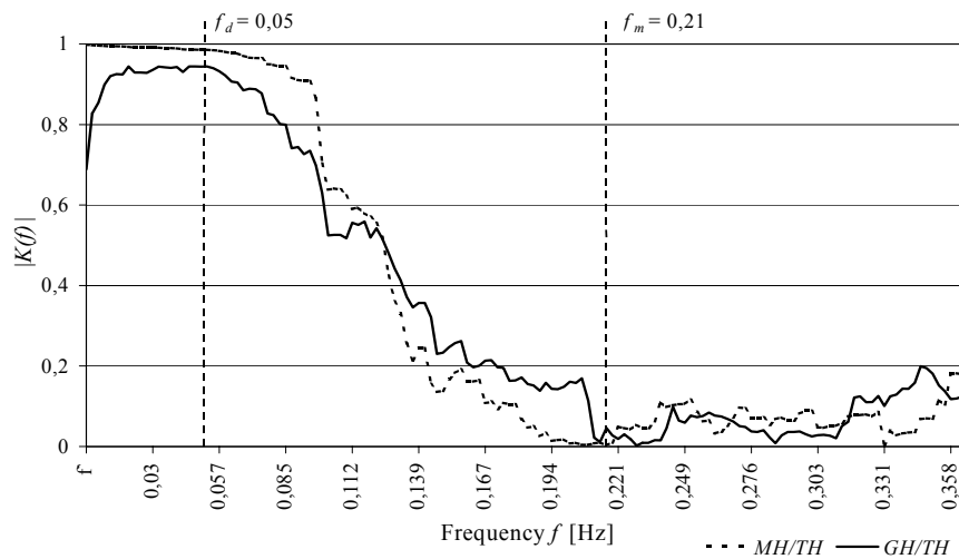
Fig. 5. Example of correlation of the course, measured with magnetic compass, with true course, and of the course, measured with gyrocompass, with true course.
