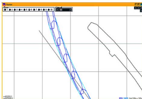
Fig. 1. A ship's movement path as a sequence of consecutive ship's hull positions (bird's eye view)
