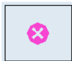
Fig. 2. Isolated danger of depth less than the safety contour: wrecks, obstructions, under water rocks [4]
