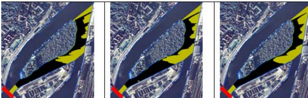
Fig. 9. Results of modified viewshed analysis for spline, natural neighbor and kriging DSM [own study]
