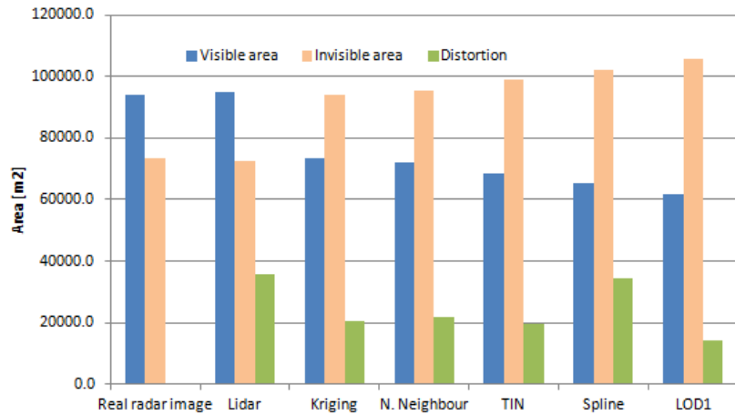
Fig. 11. Comparison of visible and invisible areas for studied DSMs [own study]
